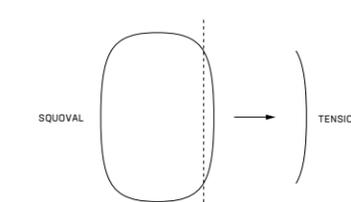
Inspired by the surface tension of water, this element gently reflects light and invites interaction. This detail adds a controlled yet dynamic element to an otherwise flat surface. Like the edge of a samurai’s sword, it is precise, elegant, and beautiful. The form has an embedded function and acts as a guard to water; its symmetrical incline gently repels liquid.
