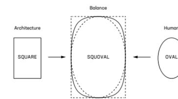
A hybrid shape created from a square and an oval, which INAX has aptly named a “Squoval.” This unique hybrid geometry celebrates the friendly and human shape of the oval with the structure and architectural relevance of the square. The combination of human and architectural elements (humanitecture) helps to create a form which is both conscious of the architectural space in which it will be placed and demonstrates a sensitivity toward human interaction, connecting people and architecture.
